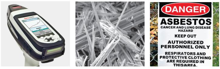
The microPHAZIR™ AS analyzer provides rapid screening of Chrysotile, Crocidolite, Anthophyllite, Tremolite, Actinolite, and Amosite.
