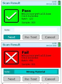
Once a measurement is complete, the analyzer provides a clear PASS/FAIL result within seconds.
