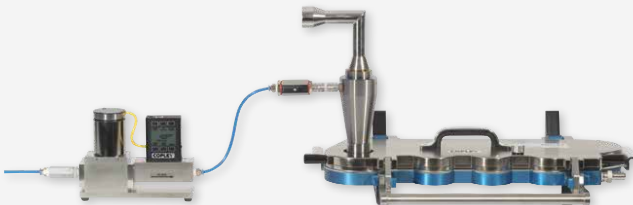
↑ Next Generation Impactor (NGI) fitted with Mixing Inlet, Compressed Air Flow Controller and Inlet Manifold for constant low flow rate tests, such as paediatric studies
