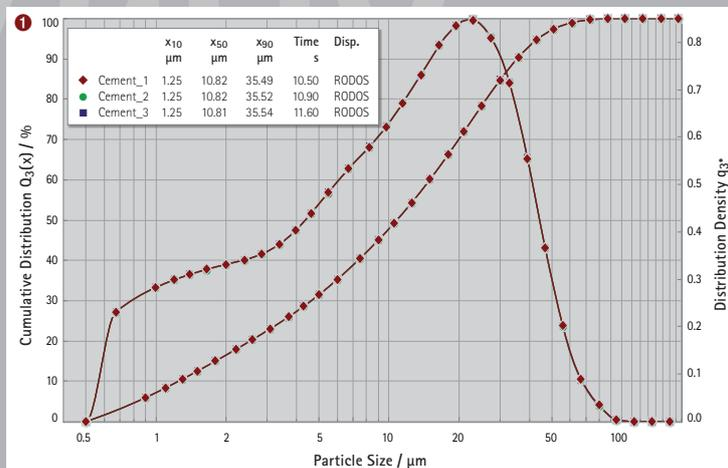
① Cement: bimodal (0.5 μm to 150 μm; x<sub>50</sub>-value @ 10.82 μm). With measuring times of 11 ± 1 seconds
