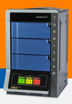
Multi-sample Accelerated Stability Analyzer
