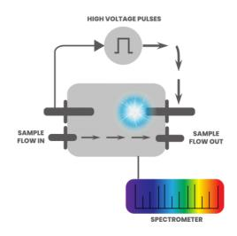
Measuring the atomic emission spectrum enables quantitative analysis of the metals contained in the sample.
