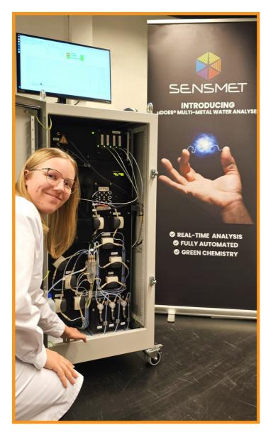
The Sensmet µDOES® Analyser is a cuttingedge online instrument that precisely quantifies dissolved metal concentrations in aqueous solutions.
