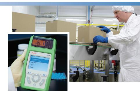
The Thermo Scientific™ TruScan™ GP analyzer is the latest in our TruScan family of handheld Raman spectrometers for raw material identification and finished product inspection.
